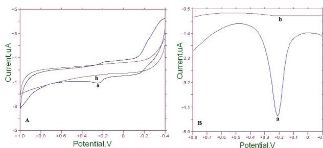
Figure 1. (A) CVs of GSH and (B) DPVs of GSH in PBS (pH 7.4) at (a) SWCNT/GCE modified sensor and (B) bare GCE vs. Ag/AgCl.
